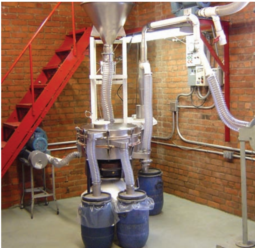
This small lab is a controlled environment for materials that require extreme purity or clean conditions. A 14-inch tumbler screener is shown processing material.
